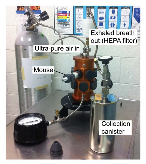
Figure 1. Assembled apparatus for collection of exhaled breath samples from groups or individual mice. Selected components of the apparatus are indicated. doi:10.1371/journal.pone.0069802.g001
