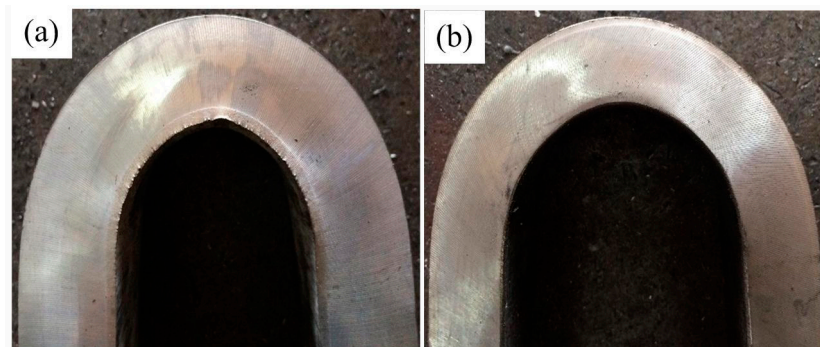
Figure 13. Bending test of the titanium clad steel plate with Nb interlayer: (a) Inner bending; (b) Outer bending.
