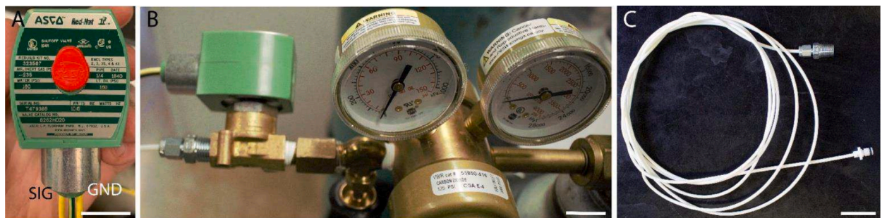
Fig. 7. Photographs of gas-delivery mechanism. A) A solenoid valve and the associated wiring scheme, including the signal (SIG, 12 V from the relay) and the ground (GND). B) The solenoid valve is attached to the gas tank regulator using a straight brass adaptor. C) The assembled polyurethane tubing is connected to the solenoid valve with the Yor-lok fitting and is connected to the chamber with the quick-disconnect coupling. The scale bars represent A) 17.5 mm, B) 21 mm, and C) 6.35 mm.
