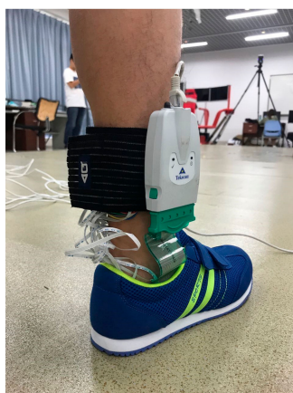
Figure 4. Both the lower-shank mounted block of the instrumented insole and the signal box of the F-scan system were attached to the lower-shank.
