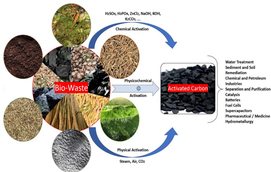
Figure 6. Schematic clarification of activated carbon derived from bio-waste and its potential uses.
