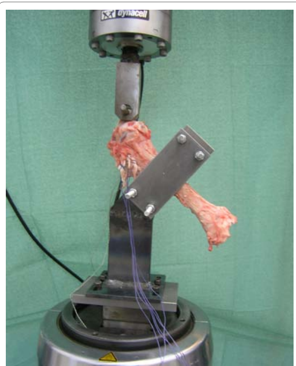
Figure 1 Test arrangement. Specimen adaptation to the Servohydraulic Fatigue System (Universal Testing Machine Instron® 8800) with a special fixture designed for this purpose.
