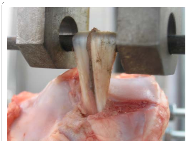
Figure 2 Elongation of tendons without pull-out. When no pull-out was observed, tendons suffer elongation as fibers begin to fail.
