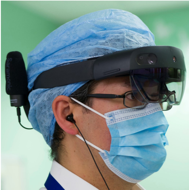
Figure 1 Microsoft HoloLens 2 worn around the head with an external microphone attached.
