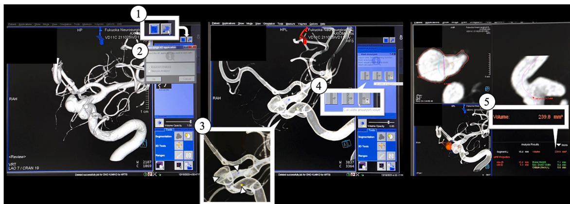
Fig. 1. Method of using the simplified volume calculation function in the cerebral angiography system and flat-panel detectors (Artis Q BA Twin; Siemens AG, Forchheim, Germany).
