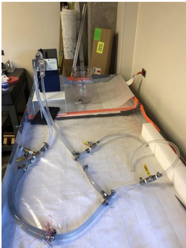
Fig 1. Finalized flow loop holding 1 L of Ringer's lactate (RL) solution.
