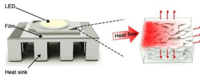
Figure 6. Schematic diagram of heat conduction in a BN film. Adapted with permission [44], Copyright 2021, Applied Nano Materials.
