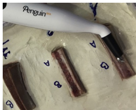
Figure 4 Implant stability measure by a Penguin RFA device.
