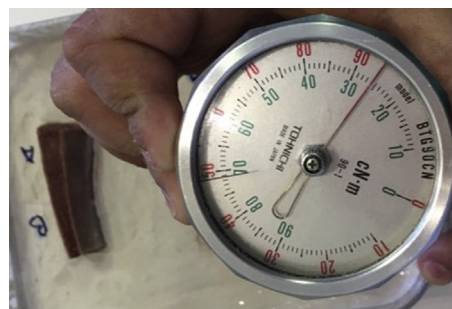
Figure 3 Implants placed using a calibrated torque wrench.
