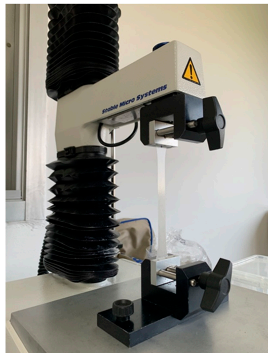
(b) Analysis of the mechanical property of the film on the texture analyzer
