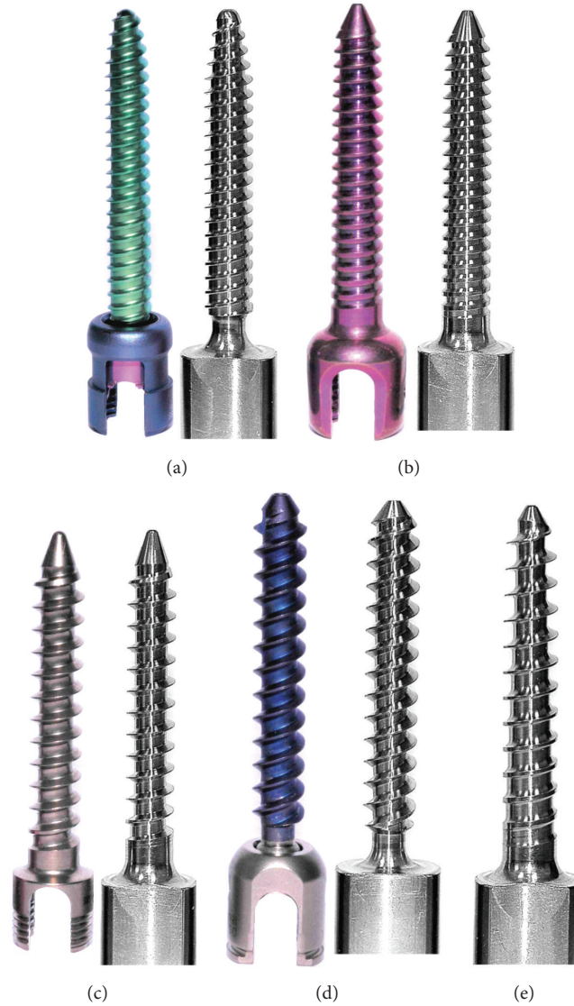
FIGURE 5: Tested pedicle screws: (a) Synthes, (b) A-Spine, (c) Moss Miami, (d) Viper, and (e) Optimal.
