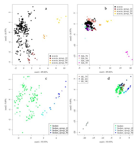
**Figure 2.** Results of electronic tongue linear discriminant analysis (LDA) models for the classification of authentic and adulterated acacia (**a**) (n = 381) and linden (**c**) (n = 148) honeys and independent prediction of EUnonEU blends for acacia (**b**) (n = 381 + 66) and linden (**d**) (n = 148 + 59) honeys; • training, × validation and ▲ independent prediction.
