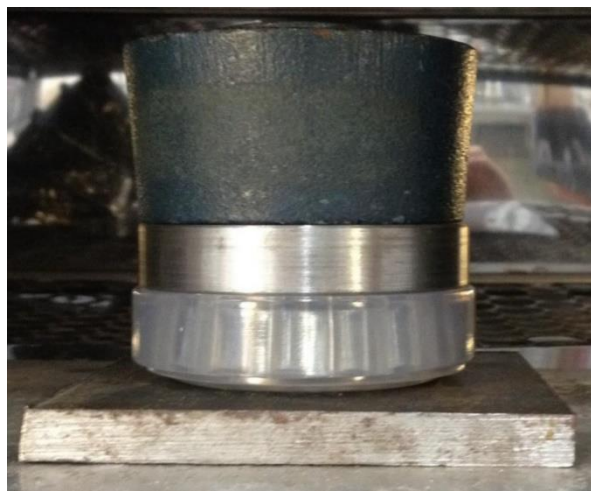
Figure 2. Freezing of stresses-prototyped model in stereolithography.
