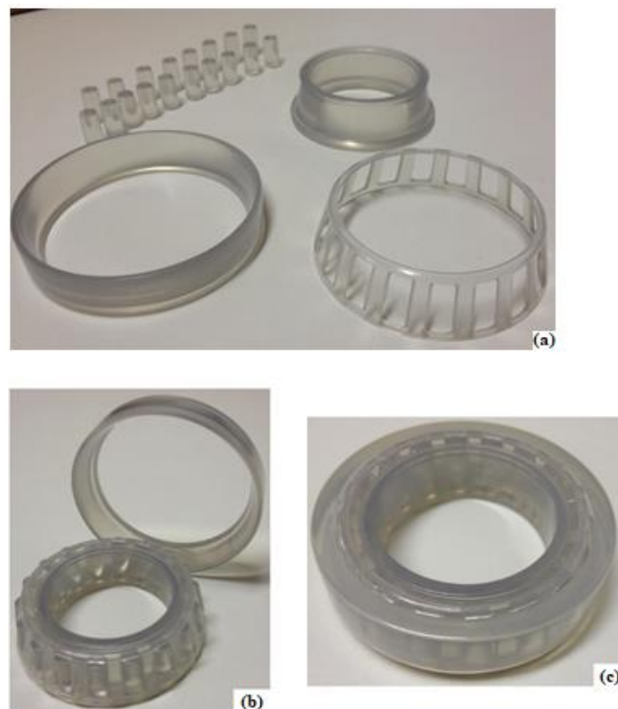
Figure 1. (a) Sample of tapered roller bearing made in stereolithography (SLA)-separate components. Sample of tapered roller bearing made in stereolithography (SLA): (b) separate outer ring, and (c) mounted bearing.
