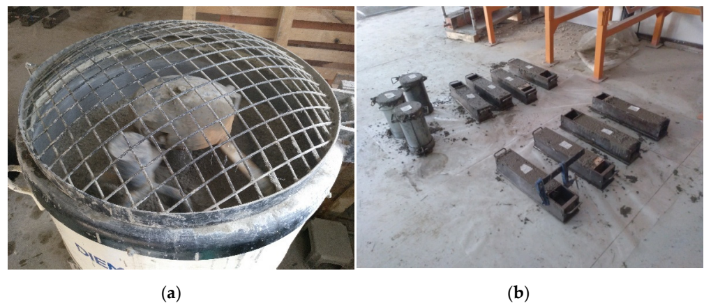
Figure 2. (a) Production of concrete and (b) specimens produced in a batch of this program.
