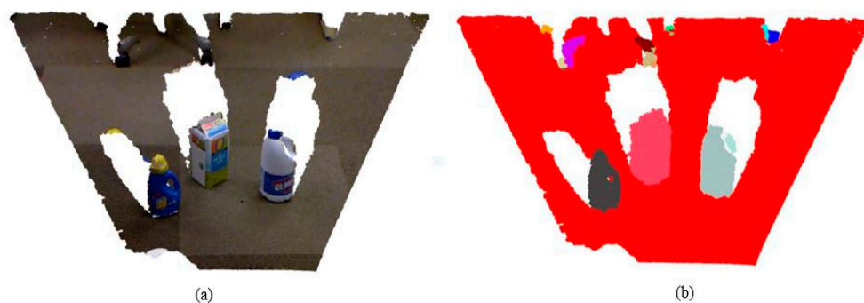
Figure 9. The segmentation result of our method on a point cloud containing a table surface and several objects (bottles and boxes): (a) the original point cloud with real colors, and (b) the segmentation result with different objects labeled in different colors, respectively.
