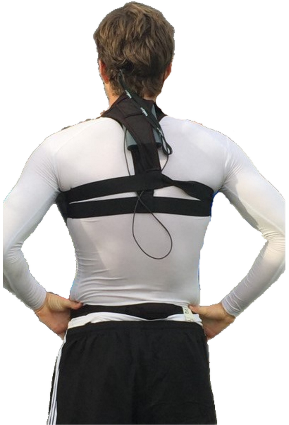
Fig 1. The Tobii Pro Glasses 2 recording unit attached on the upper back of one of the participants. Printed with permission.
