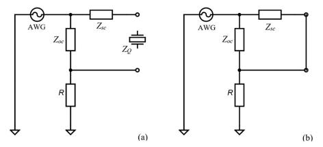
**Figure 4.** Standard method for impedance compensation. (a) Open-circuit compensation. (b) Short-circuit compensation.
