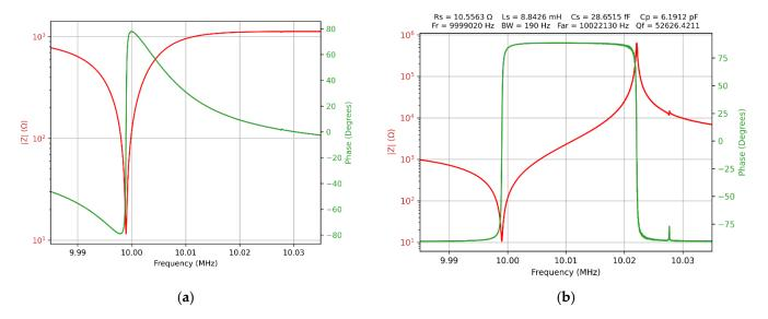
**Figure 6.** Bode plot of the raw data for a QCM sensor in the air with balun transformer topology. (a) Without compensation. (b) With compensation.
