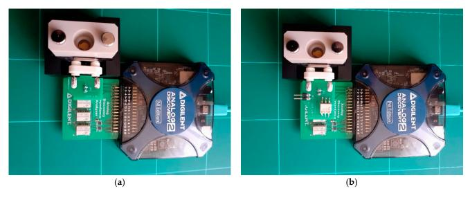
**Figure 2.** QCM versions based on virtual impedance analyzer. (a) Half-bridge configuration for wide dynamic range. (b) With one grounded electrode based on a balun transformer.
