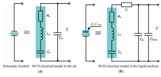
Figure 3. Butterworth–van Dyke (BVD) model of the QCM sensor. (a) In the air. (b) In the liquid medium.
