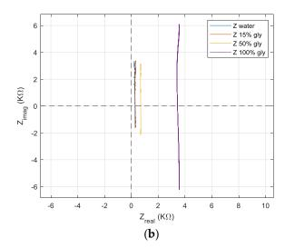
**Figure 9.** QCM sensor in water, in two concentrations of the glycerin-water solution, and in glycerin after advanced shunt and stray capacitance compensation. (a) Bode plot. (b) Nyquist plot.
