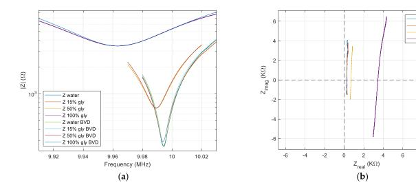
**Figure 8.** QCM sensor in water, in two concentrations of the glycerin-water solution, and in glycerin after real-time shunt and stray capacitance compensation. (a) Bode plot. (b) Nyquist plot.
