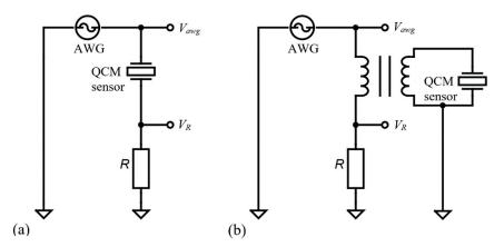
**Figure 1.** Methods of the impedance analysis. (a) Half-bridge configuration for wide dynamic range. (b) With one grounded electrode based on a balun transformer.
