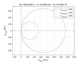
**Figure 5.** Simulation of the residual shunt and stray capacitance effect as Nyquist plot considering the liquid medium.
