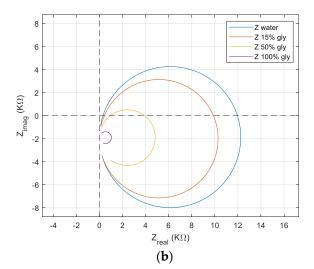
**Figure 7.** Nyquist plot for QCM sensor. (a) In water and air. (b) In water, in two concentrations of the glycerin-water solution, and in glycerin.
