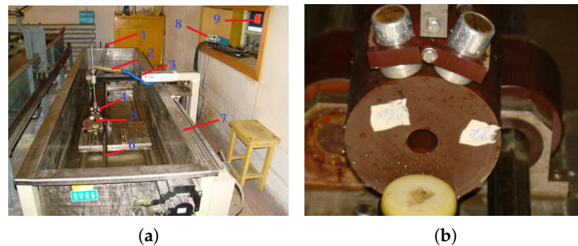
Figure 9. Appearance of testing equipment ((a) testing equipment: 1. rotary encoder, 2. water pipe, 3. detection cantilever, 4. transmitting and receiving transducers, 5. solid propellant, 6. mechanical transmission link, 7. water tank, 8. transmitter/receiver unit, and 9. industrial computer), (b) transducer and propellant).
