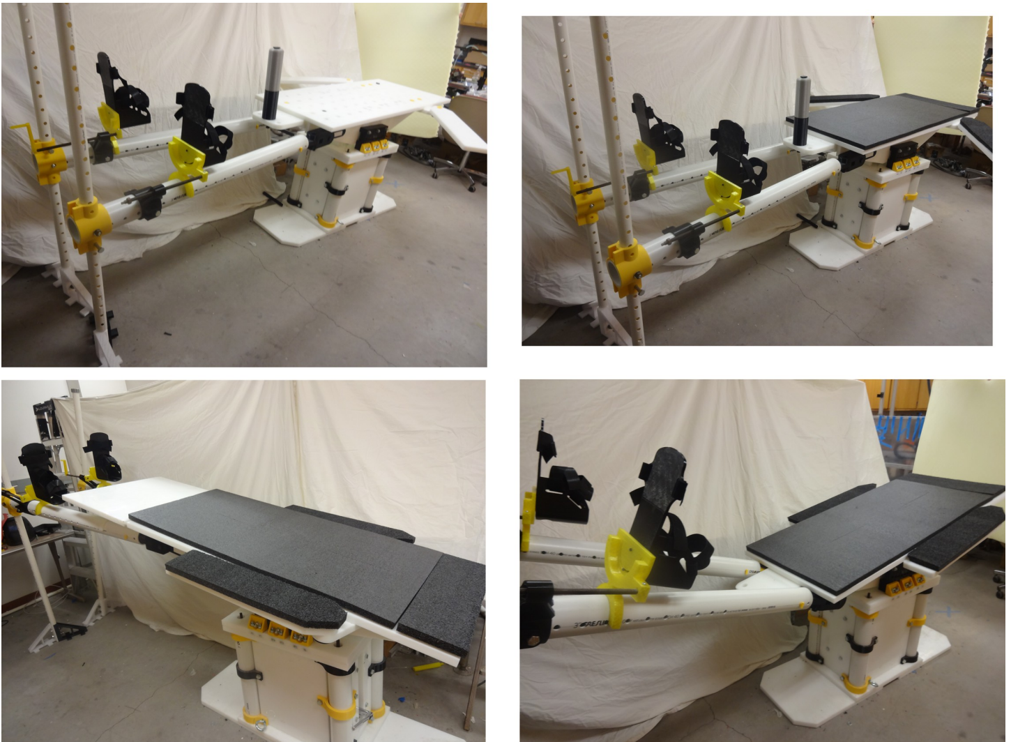
Fig 28. a) The final assembly with no pads. b) The final assembly with pads flat. c) The final assembly with pads tilted towards head (Trendelenburg position). d) The final assembly with the pads tilted towards feet (reverse Trendelenburg).
