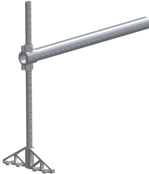
Fig 24. Addition of both vertical_pvc_leg_support_new to 1.25in pipe.
