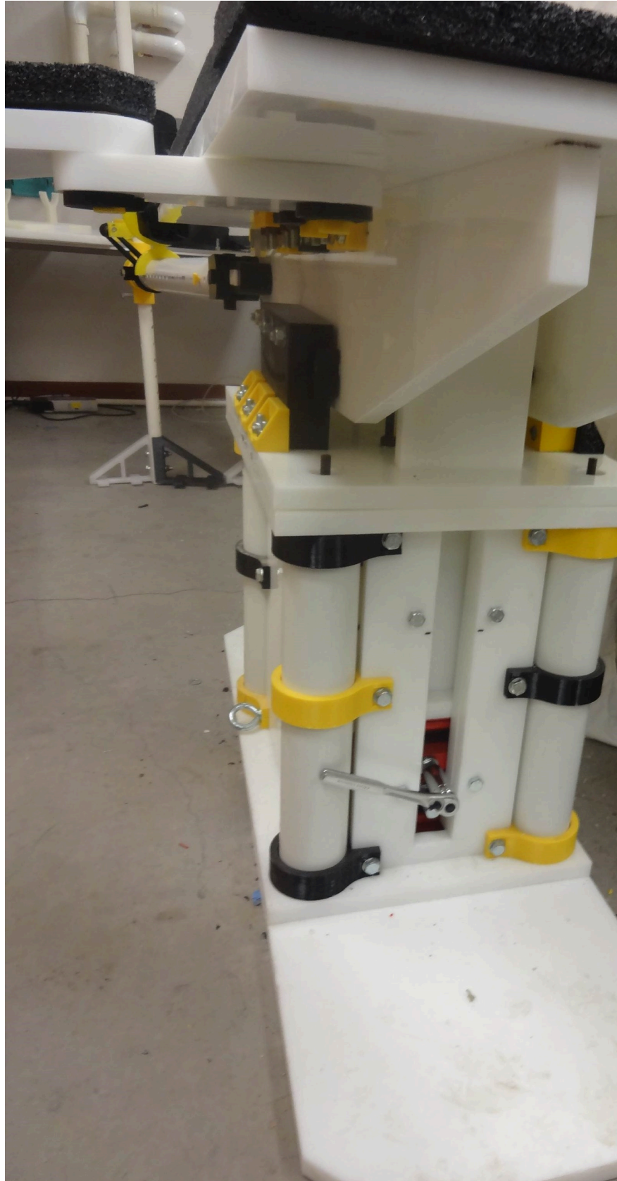
Fig 29. Details of wrench used to control heights of motor cycle jack and thus the table surface.
