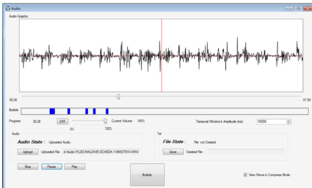
Figure 4. Module used to review audio, detect bubbles, and save the results in a text file.
