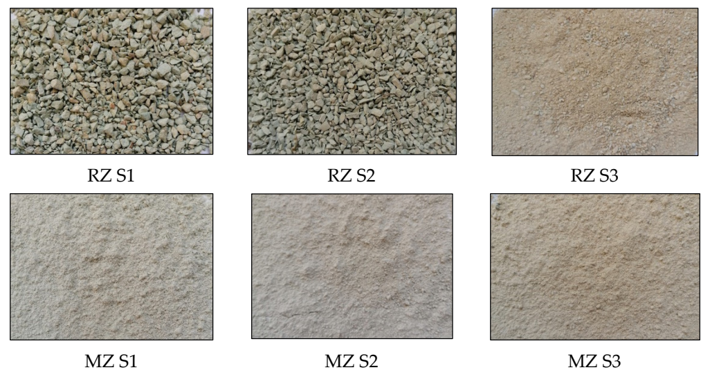
Figure 1. Zeolitic volcanic tuffs before (RZ S1, RZ S2 and RZ S3) and after micronization (MZ S1, MZ S2 and MZ S3).
