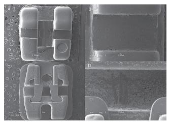
Figure 3 - Steel and elastomeric-tied brackets (A), magnified slot (B); self-ligating bracket (C), magnified slot (D).
