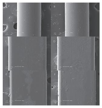
**Figure 2** - Wires before and after friction, respectively: 0.016-in NiTi wire (A and B),  $0.016 \times 0.021$ -in NiTi wire (C and D) and  $0.019 \times 0.025$ -in stainless steel wire (E and F).
