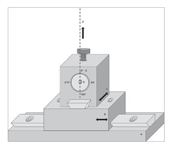
**Figure 1** - Testing appliance design: base locked to the testing machine (**A**), horizontal movable bases for bracket/wire alignment (**B** and **C**), bracket bonded to plastic pedestal (**D**), 360-degree display (**E**) and wire specimen attached to the load cell (**F**).
