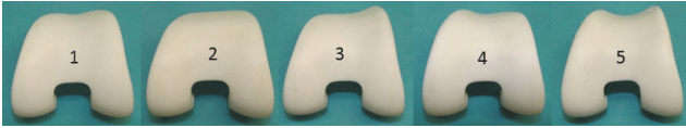
FIGURE 2: Design variations of Genesis II endoprosthesis with modified patellofemoral groove: (1) original design, (2) being flat, (3) being medially high, (4) being laterally high, and (5) both sides high.
