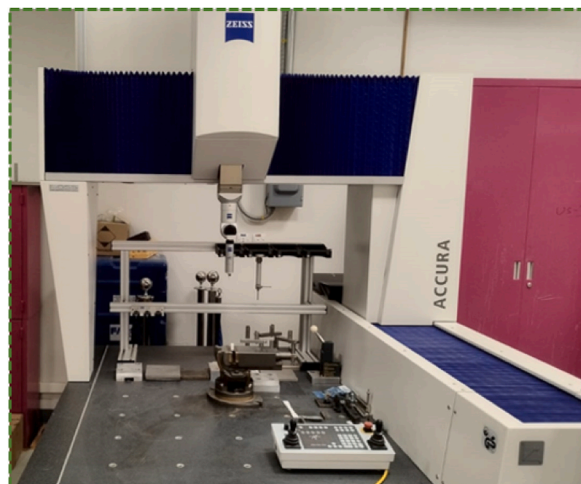
Fig. 7. CMM set up deployed to measure the 3D printed parts.
