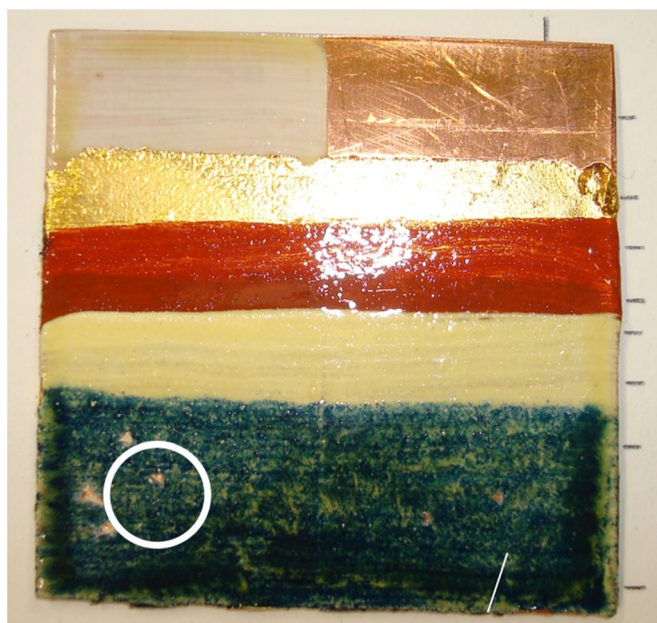
Figure 5. Photo of the paint layer sample. The white circle indicates the measurement area (reprinted with permission from Ref. 27).
