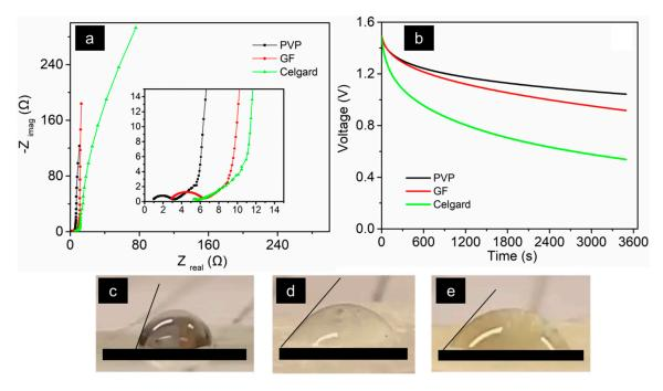
**Figure 8.** (a) Nyquist plot of the MSCs (same devices as in Figure 7). (b) Open circuit voltage (OCV) decay over time. The measurements used an AC electrode, 1-ethyl-3-methylimidazolium acetate (EmImAc) ionic liquid electrolyte, and three different separators. (**c**–**e**) The optical images used for the preliminary contact angle measurements of PVP, Glass fiber, and the Celgard separators, respectively.
