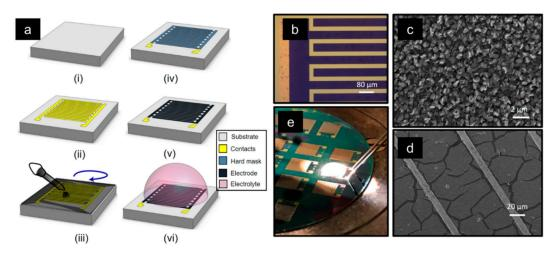
**Figure 2.** (a) Schematic CMOS compatible process for MSC fabrication. (b) Optical micrograph of the fabricated intedigitated reduced graphene oxide (rGO) electrodes on Au/Ti current collectors. (c) Graphical SEM image of vertical graphene on a 50 mm diameter Si/SiO<sub>2</sub> wafer with Au/Ti collectors. (d) SEM image of rGO on Fe/Ti/Au current collectors. (e) Electrochemical test setup of fabricated rGO-MSCs with H<sub>3</sub>PO<sub>4</sub>/polyvinyl alcohol (PVA) electrolyte.
