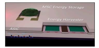
**Figure 10.** Schematic of a potential future self-powering system consisting back end of the line (BEOL) integration of an microsupercapacitors (MSC) and harvester with application specific integrated circuit (ASIC) components.
