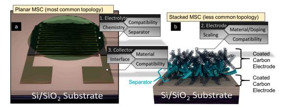
**Figure 1.** Schematic of a microsupercapacitors (MSCs)—planar (**a**) and stacked (**b**)—and its design parameters. There are 3 primary areas for performance improvement—electrolyte, electrode, and current collector. Each of these areas have 3 subset groups for improvement. This work aims to provide an overview of each area and subset group.
