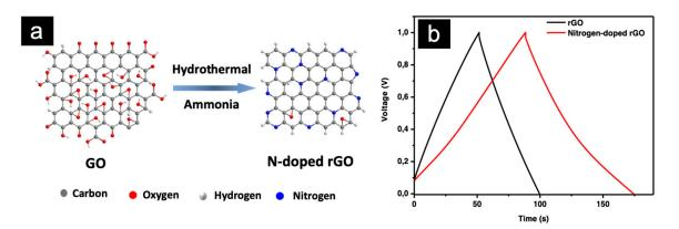
**Figure 5.** (a) Preparation of nitrogen-doped rGO from graphene oxide (GO) and ammonia solution (as the nitrogen precursor) through a hydrothermal process; (b) a galvanostatic charge–discharge (GCD) plot of rGO and a nitrogen-doped rGO.
