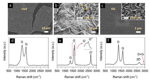
**Figure 3.** SEM images of (**a**) rGO, (**b**) carbon nanotubes (CNT), and (**c**) a vertical graphene (VG) layer as electrode materials on an SiO<sub>2</sub> surface. Insets show higher magnification of the respective sample. Raman spectroscopy images of each material are shown in (**d**), (**e**), and (**f**), respectively.
