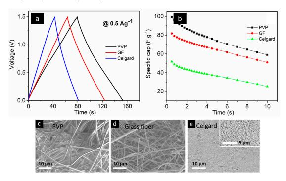
**Figure 7.** Measurements of supercapacitor devices including (**a**) GCD plots and (**b**) capacitance variations at different current densities. The measurements were done on an MSC with an AC electrode, a 1-ethyl-3-methylimidazolium acetate (EmImAc) ionic liquid electrolyte, and three different separators. (**c-e**) SEM images of polyvinylpyrrolidone (PVP), Glass fiber, and Celgard separators, respectively.
