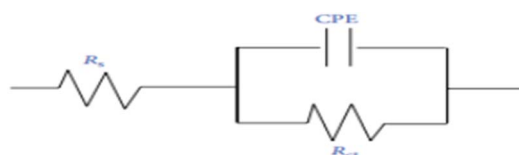
Fig. 4 Electrical circuit equivalent at the carbon steel/HCl electrolyte contact.
