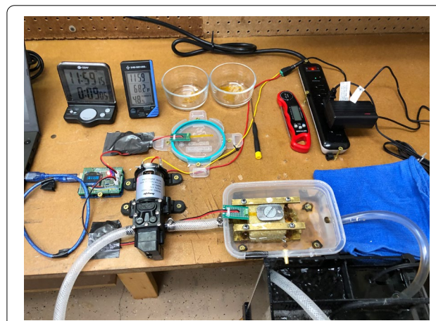
Fig. 2 Cement curing and testing station
