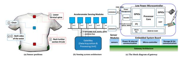
**Figure 1.** Design of wearable instrumented vest for posture monitoring: (**a**) the sensor positions (dotted lines indicate the sensors at the back of the vest); (**b**) system architecture of the multichannel accelerometer-based sensing system; and (**c**) block diagram of sensing system gateway.
