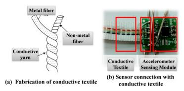
Figure 2. Conductive textile: (a) fabrication schematics; and (b) integrated with sensing module.
