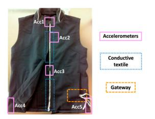
Figure 3. The fully developed wearable instrumented vest.
