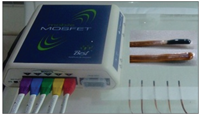
Figure 1: Photograph of mobile metal oxide semiconductor field effect transistor dose verification system
