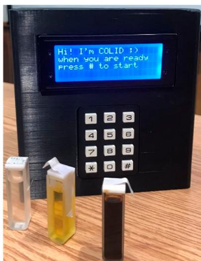
Figure 6. Final version of the device.
