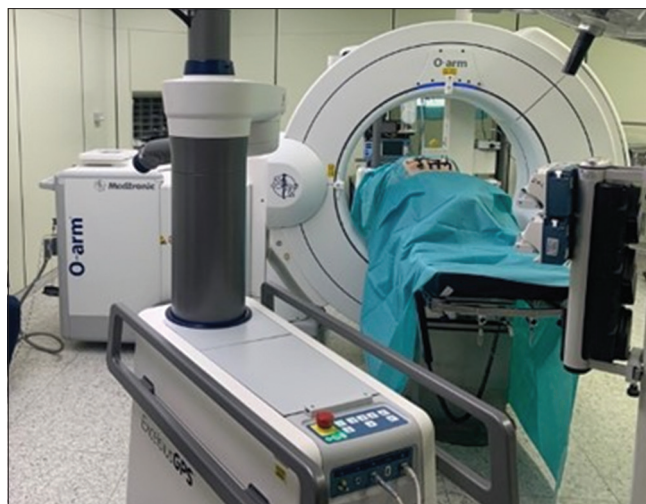
Figure 4: Surgical theater showing the combined use of the ExcelsiusGPS® Robotic Navigation Platform (left) and intraoperative cone-beam computed tomography guidance (O-arm II, Medtronic) (right)
