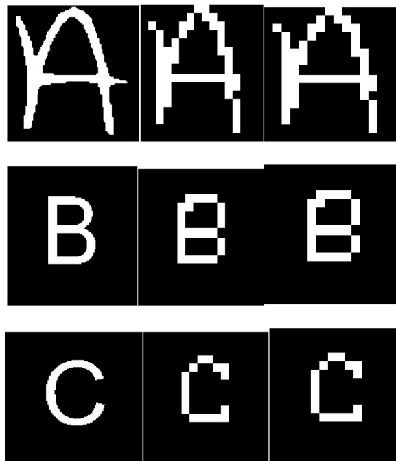
Fig. 11. Converting the spike trains generated from RGC and LRGC models within the retinal pathway into an image with 16 x 16 pixels. The first column shows the 128x128 pixel images given as input to the retina path. The second column is reconstructed images with 16 x 16 pixels from 16 x 16 spike trains which these spike trains are generated from the original ganglion cell model (RGC). The third column is reconstructed images with 16 x 16 pixels from 16 x 16 spike trains which these spike trains are generated from the proposed ganglion cell model (LRGC).
