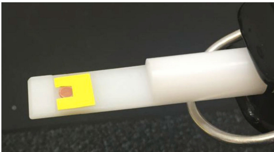
Fig. 2. ESPnano key with an affixed copper mesh TEM grid.
