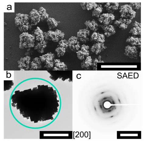
**Figure 1.** Analysis of NiHCF mesocrystal morphology. (a) SEM micrograph of NiHCF mesocrystals. (b) TEM micrograph of an individual NiHCF mesocrystal. (c) SAED pattern that corresponds to the individual mesocrystal (Diffraction area indicated by the green square; view from [200] zone axis). Scale bars:  $5.0 \, \mu m$  (top),  $1.0 \, \mu m$  (bottom left) and  $5.0 \, nm^{-1}$  (bottom right).
