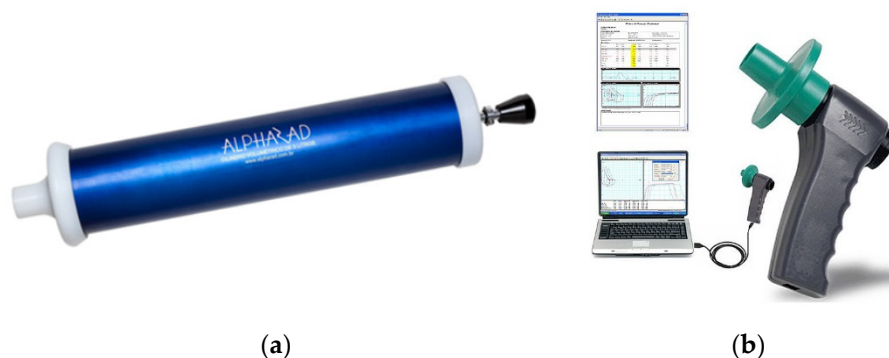
Figure 3. Components for calibrating the spirometer: (a) Calibration syringe; (b) Koko flow spirometer model 313105.
