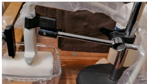
Fig. 1. Complete system implemented for vibrating the constructed phantoms.
