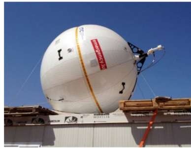
Figure 3. B-LiFE deployment in N’Zerekore, Guinea: view of the satellite communication antenna (2.4 m inflatable Ground Antenna Transmit and Receive (GATR); www.gatr.com , accessed on 17 February 2021, obtained from–SES–Société Européenne des Satellites, Betzdorf, Luxembourg) placed on the roof of the B-LiFE command and control shelter.
