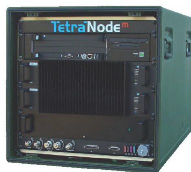
Figure 9. Bio-Garden exercise: Rohill TetraNode equipment (TETRA base station) tested during the exercise.
