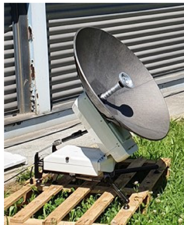
Figure 14. B-LiFE deployment in Turin, Italy, during the COVID-19 crisis: installation of the GovSat Scorpion MP80X SatCom terminal.
