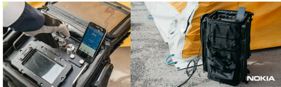
Figure 10. Bio-Garden exercise: Nokia Ultra Compact Network LTE system (LTE portable base station) tested during the exercise.
