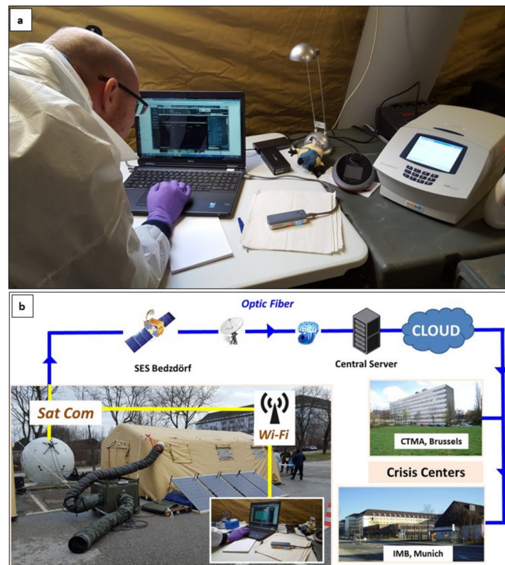
Figure 4. Exercise “Clueless Snowman” in the Institute of Microbiology, Bundeswehr, Munich: (a) Use of the MinION sequencer (ONT) in the B-LiFE facility during the exercise “Clueless Snowman”; (b) MinION data flow from the laboratory to the tent to the crisis centre.
