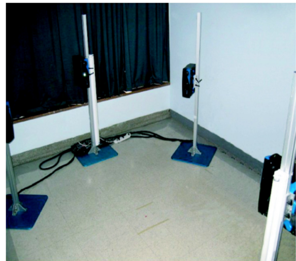
Figure 1 Inspeck system. Inspeck system used for capturing surface topography data. Four digitizers allow the capturing of the full surface of the patient torso.
