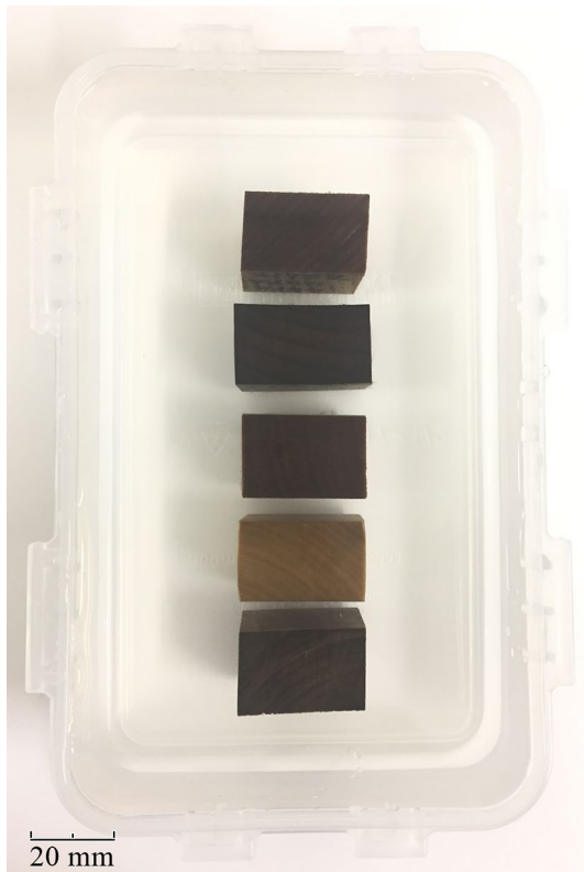
Fig. 1 The photograph shows the FA-diffusivity value phantom. The pieces of wood were placed in a container of distilled water that was pressed and fixed with a lid. Five kinds of wood, 20 mm×30 mm×30 mm in size, were boiled in distilled water, and the distilled water penetrated into the interior. The wood types are Gleditsia triacanthos , Cinnamomum sieboldii , Euodia meliifolia , Ilex pedunculosa , and Acer palmatum (from top to bottom)
