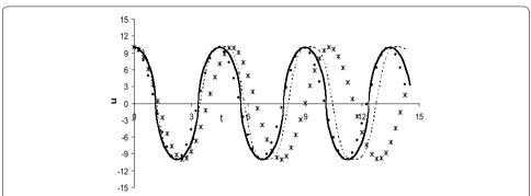
**Fig. 2** Comparison of the analytical approximate periodic solution obtained by present method (denoting by *circles line*) with numerical solution obtained by fourth order Runge–Kutta method (denoted by *solid line*) and also with the first-order (denoted by *cross lines*) as well as second-order (denoted by *dash line*) approximations obtained by harmonic balance method (Wu et al. 2003) for  $\alpha = \beta = 2$ , A = 10
