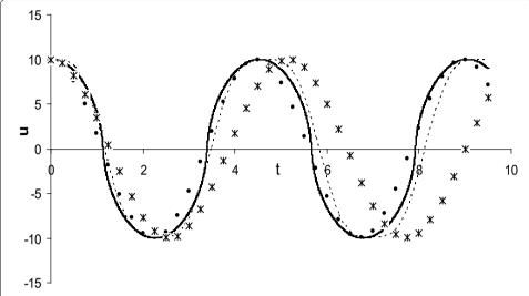
**Fig. 1** Comparison of the analytical approximate periodic solution obtained by present method (denoting by *circles line*) with numerical solution obtained by fourth order Runge–Kutta method (denoted by *solid line*) and also with the first-order (denoted by *cross lines*) as well as second-order (denoted by *dash line*) approximations obtained by harmonic balance method (Wu et al. 2003) for  $\alpha = \beta = 1$ , A = 10
