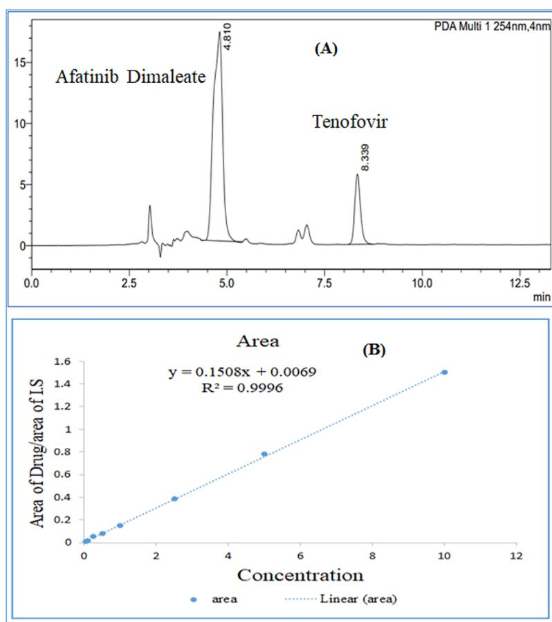
Figure 9. HPLC chromatogram of internal standard (Afatinib Dimaleate) and tenofovir. (A) Calibration plot (B).
