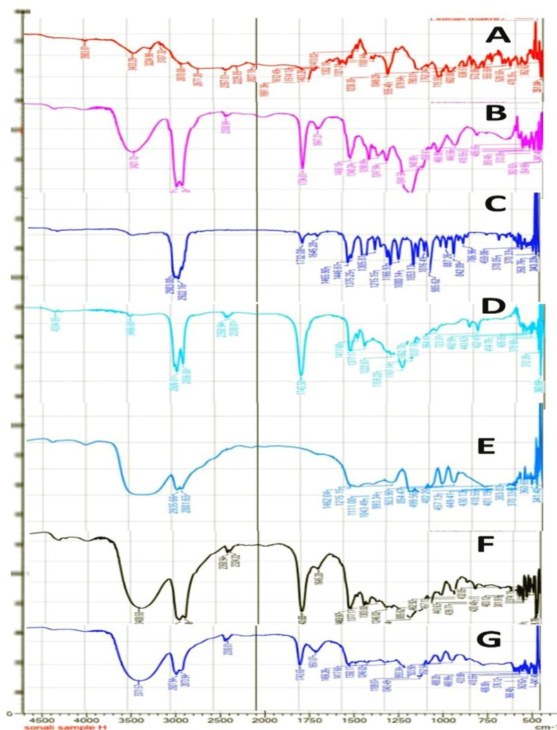
**Figure 3.** FT-IR spectra of pure tenofovir (A), eucalyptus oil (B), Kolliphor EL (C), Kollisolve MCT 70 (D), glycerol (E), physical mixture (F), and TNF-SEDDS F6 (G).
