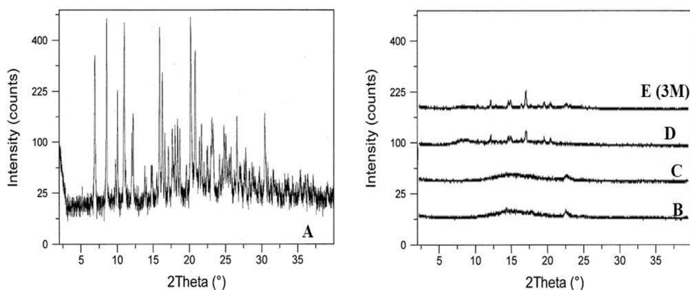
**Figure 5.** XRD spectra of tenofovir drug (A), Kolliphor EL (B), Kollisolv MCT 70 (C), TNF-SEDDS F6 (D), TNF-SEDDS F6-3 M (after 3 months) (E).
