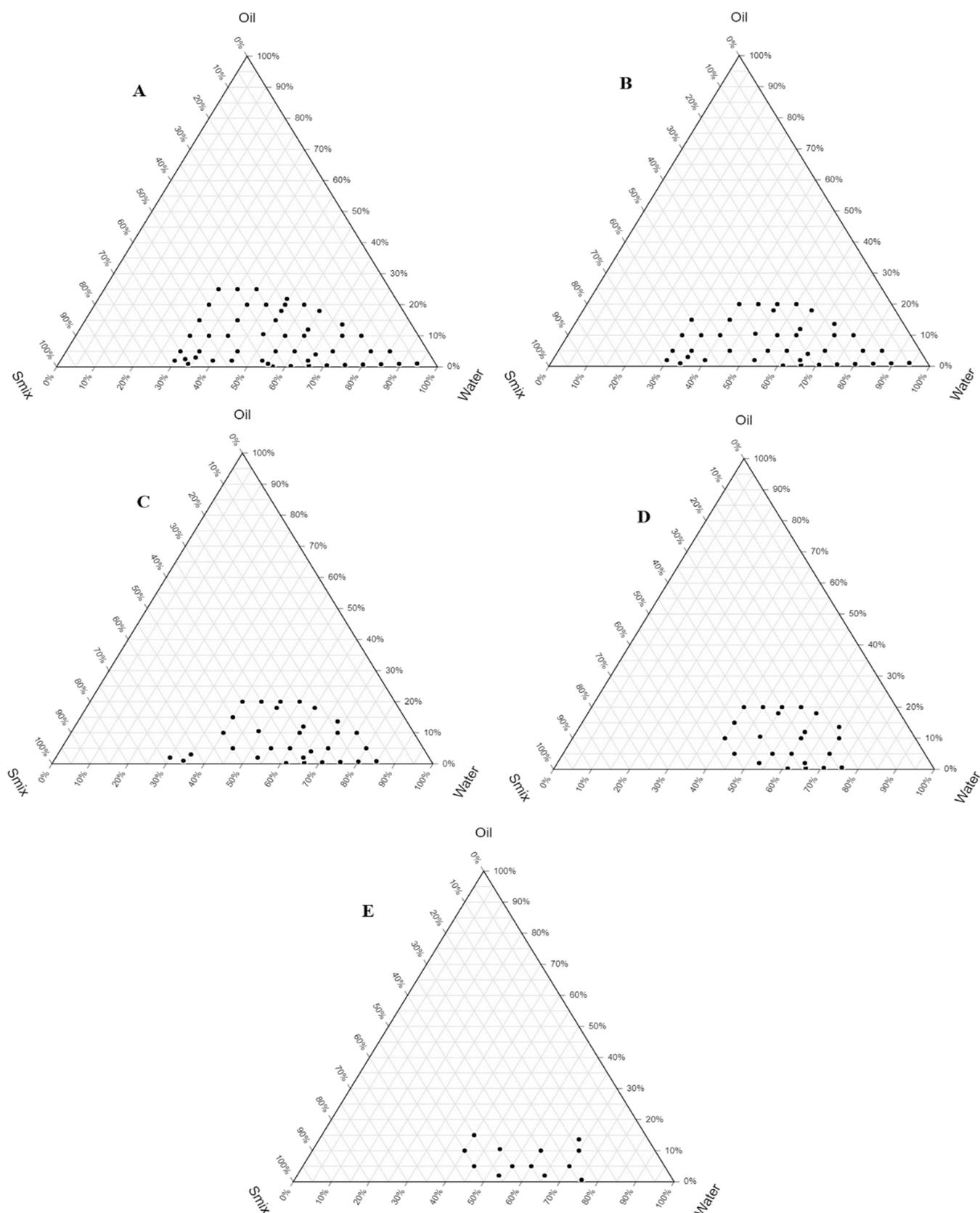
**Figure 1.** Pseudoternary phase diagram for  $S_{\text{mix}}$  (A = 3:1, B = 2:1, C = 1:1, D = 1:2 and E = 4:1).
