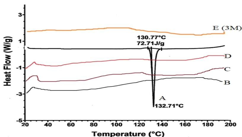
**Figure 4.** DSC spectra of tenofovir drug (A), Kolliphor EL (B), Kollisolv MCT 70 (C), TNF-SEDDS F6 (D), and TNF-SEDDS F6-3 M (after 3 months) (E).
