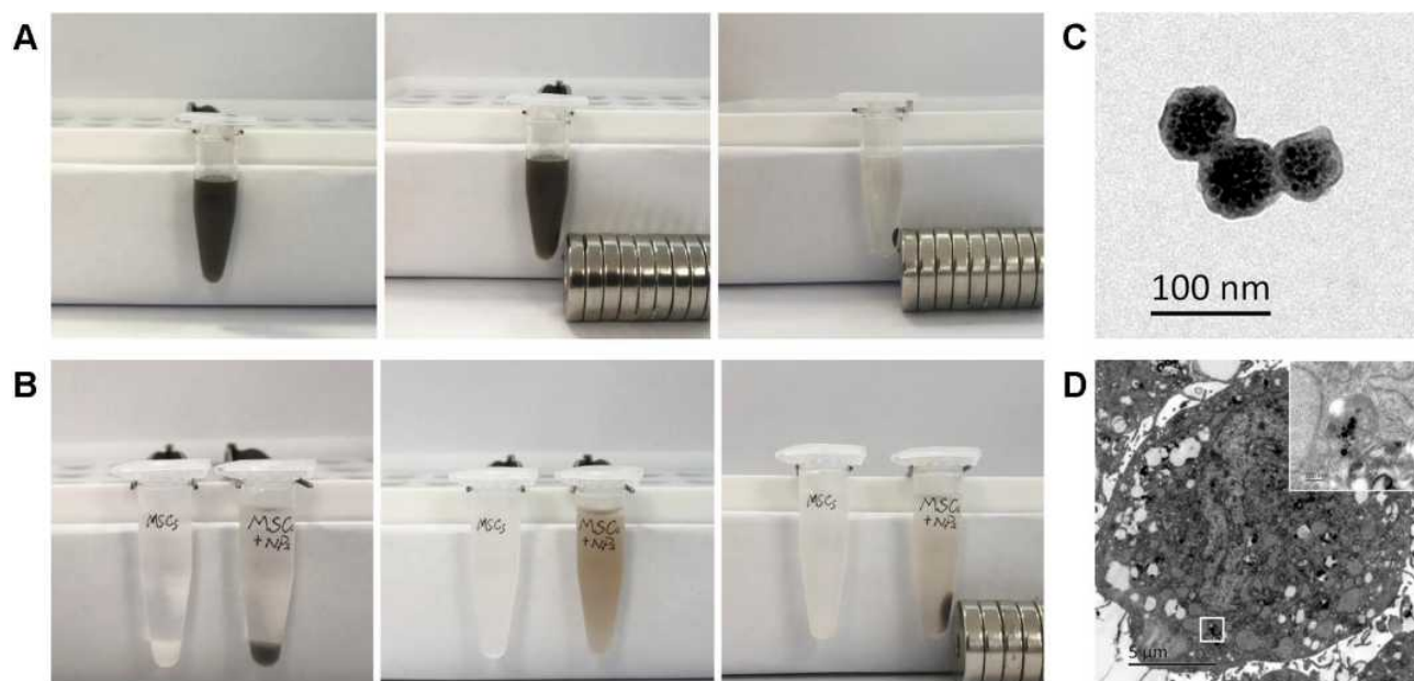
Figure 2 Morphological and magnetic characteristics of \text{Fe}_3\text{O}_4 @PDA NPs and \text{Fe}_3\text{O}_4 @PDA-labelled MSCs. (A) In the physiological saline suspension of \text{Fe}_3\text{O}_4 @PDA, the materials were attracted to the magnet side after 24 hours. (B) Saline suspension of MSCs and \text{Fe}_3\text{O}_4 @PDA-labelled MSCs, the \text{Fe}_3\text{O}_4 @PDA labeled MSCs was attracted to the magnet side at 15 min after placing the magnet. (C) Transmission electron microscope image of \text{Fe}_3\text{O}_4 @PDA. (D) Transmission electron microscope image of \text{Fe}_3\text{O}_4 @PDA-labelled MSCs (scale: 5 \mu\text{m} ) and \text{Fe}_3\text{O}_4 @PDA in endocytosis vesicles (scale: 200 nm).
