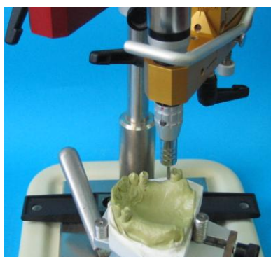
Figure 1: Formation of guiding surfaces
