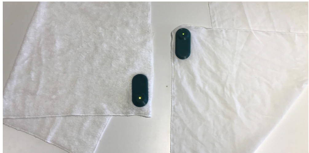
Figure 1. The conceptual prototype of Tactowel. Soft and hard textures are represented by two different towels. The soft Tactowel ( left ) is 40% bamboo-60% cotton mix bath towel and the hard Tactowel ( right ) is 100% cotton peshtemal. The green hard case is a dummy device that contains LED for participants to believe it is fully-functioning.
