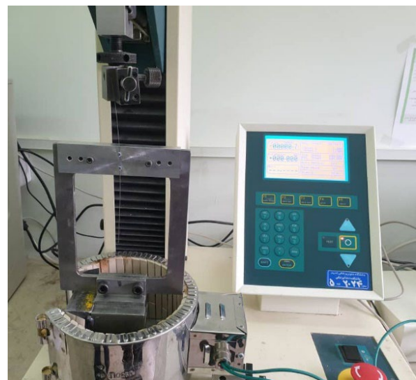
Fig. 2: Attachment of the aluminum plate to the base of the Universal testing machine. The aluminum plate was surrounded by MARDON heater
