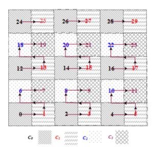
Figure 4. Slot assignment using algorithm 2 (GCA).
