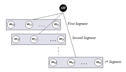
Figure 7. Segmentation architecture of member nodes inside a sector.
