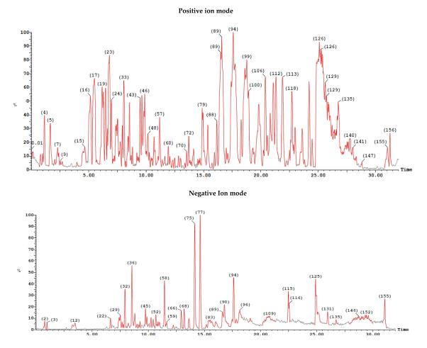
**Figure 11.** A cell-free dichloromethane extract run on both ESI-MS positive and negative ion mode for antibiotic detection from the isolate *Paenibacillus ehimensis* isolate MZ921932 using XEVO TQD triple quadrupole instrument.
